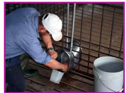
Picture 3. Measuring water flow-rate. Photo courtesy of Dr. William Hollis
